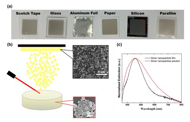
Fig. 1 a Silver nanoparticle films deposited by RIR-MAPLE onto different types of substrates. b Schematic representation of RIR-MAPLE process, in which silver nanoparticles in the target are deposited onto the substrate. The *bottom* SEM image shows the as-
