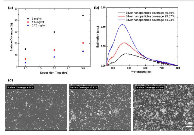
Fig. 2 a Silver nanoparticles deposited by RIR-MAPLE using different target concentration and deposition time. Each surface coverage point is obtained by averaging six SEM images, and the *error bar* represents the standard deviation of surface coverage. **b** The
