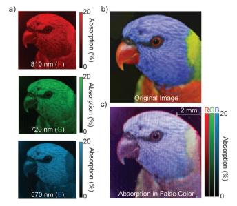
**Figure 4.** Reconstructed RGB image. a) Absorption images at the three different resonances taken with same bandpass filters as in Figure 3f. b) Original down-sampled image used to create the photomasks. c) The final reconstructed image from the three different absorption images.
