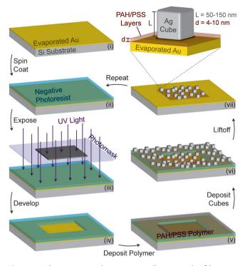
**Figure 1.** Fabrication procedure. Diagram illustrating the fabrication steps used to create multiple different self-assembled metasurface pixels on a single substrate. On the top right is a schematic of a single subwavelength absorber consisting of a silver nanocube separated from a gold substrate with a 4–10 nm polymer spacer layer.
