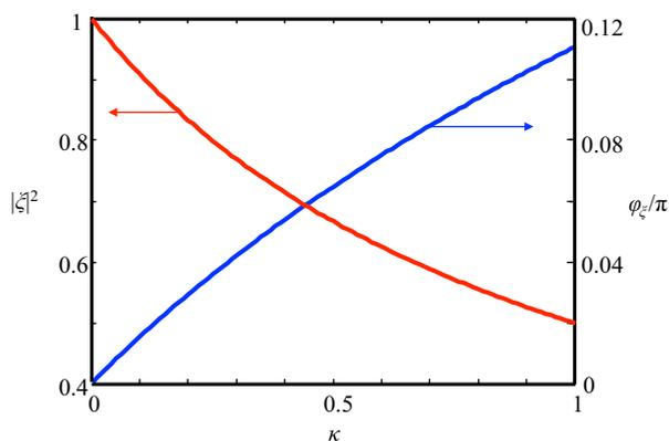
FIG. 2. (Color online) Comparison between nonlinear transmission  $|\xi|^2$  (in red) and nonlinear phase shift  $\phi_\xi$  (in blue) as a function of the dimensionless nonlinear strength parameter  $\kappa$ .
