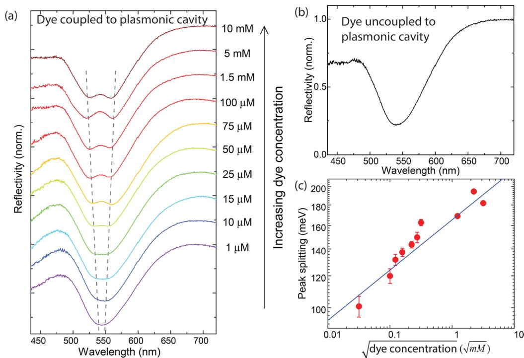
**Figure 3.** Tuning of dye concentration. (a) Reflectance spectra of dye coupled to the plasmonic cavity for varying dye concentrations. The splitting becomes larger as the dye concentration increases. (b) Reflectance spectra of dye uncoupled to the plasmonic cavity, showing a fundamental resonance at 541 nm. (c) The extracted peak splitting energy as a function of the square root of the dye concentration. The solid line is a fit to eq 2.
